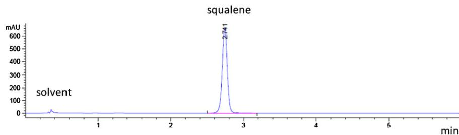
**Fig. 2.** RP-HPLC chromatogram of squalene in Bio Farma's oil-in-water adjuvant. RP-HPLC analysis is used to determine the squalene concentration in the emulsion; the area of the peak being proportional to the squalene concentration in conjunction with a known set of squalene standards.
