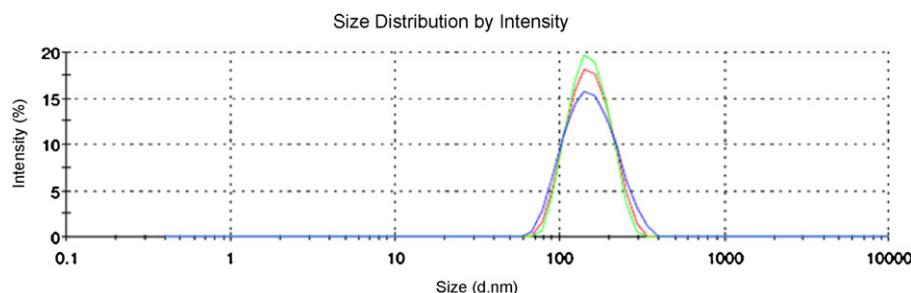
**Fig. 1.** Particle size measurement of Bio Farma's oil-in-water adjuvant. Average particle size within the emulsion as determined by dynamic light scattering (triplicate measurements of the same sample shown), indicating an average particle diameter of approximately 140 nm.
